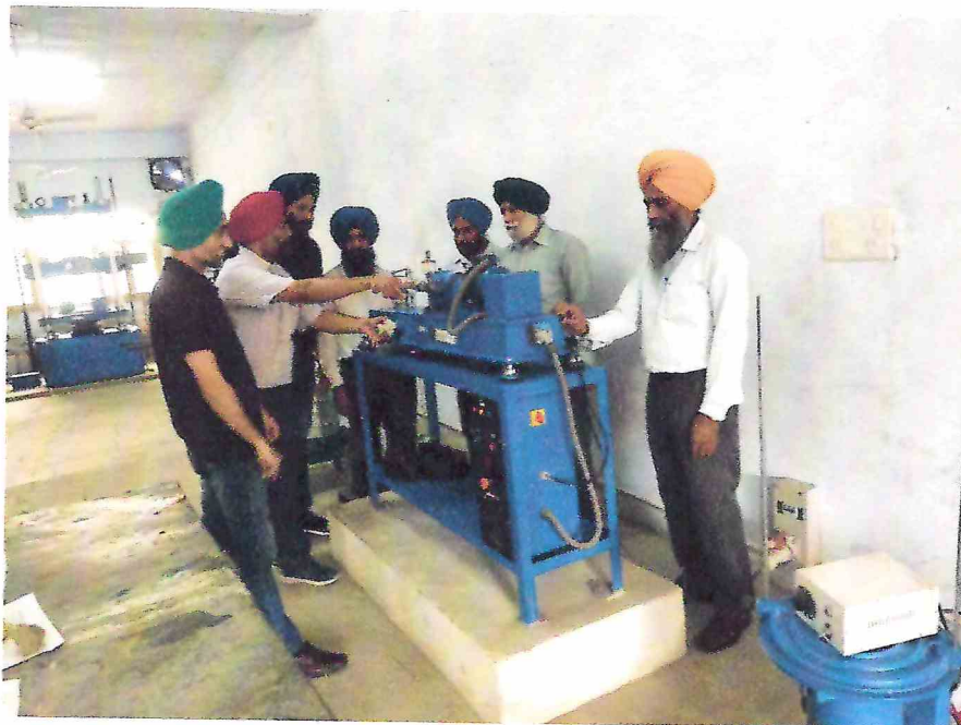
Glimpse of practical training on torsion testing machine to technical staff during SDP (20-24 Aug 2018)
